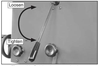
Figure 16. Quick release tension lever.
